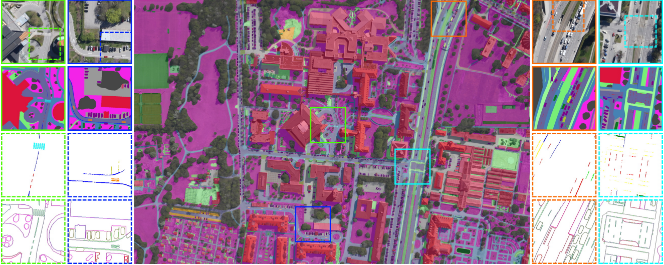
Figure 1: SkyScapes image with overlaid annotation and zoomed-in samples ( \times 2 : solid line, \times 4 : dashed line). Top to bottom: RGB, dense annotation (20 classes), lane markings annotation (12 classes), multi-class edges. Class colors as in fig. 2.
