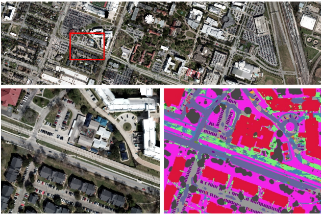
Figure 8: Results of our model trained on SkyScapes and tested on the GRSS_DFC_2018 dataset (over Houston, USA) with GSD adjustment and without fine-tuning.
