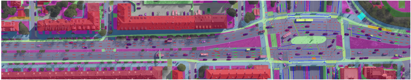
Aerial image with overlaid annotation: dense (19 classes) and lane markings (12 classes); the dataset covers 5.7 km 2 .
